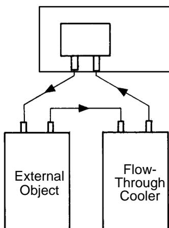
With immersion and flow-through coolers from Thermo Haake, the heat transfer liquid can be cooled down considerably below 0°C and the circulator can be rendered independent of tap water.
