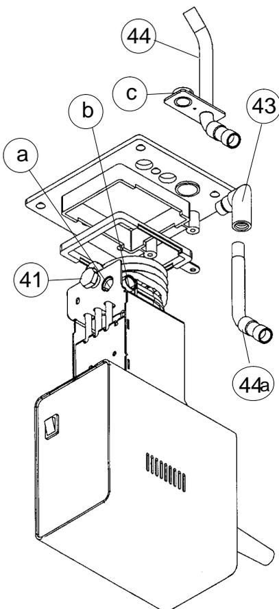
Mount the temperature control module with plate to the bath bridge.
