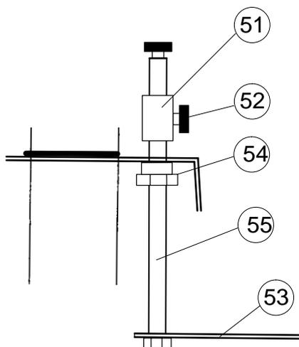
The height adjustment of the lifting platform is carried out via the thumbwheel screws **52**.
