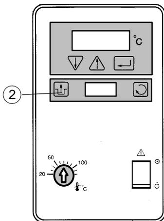
Quite often closed external systems cannot be prefilled as suggested. In this case the internal bath of the unit has to be filled to the max. level. After starting the unit, the pump will feed the necessary liquid to the external system. Should the demand be higher than the volume difference between high and low, the low liquid level sensor will be activated and the pump switched off.
