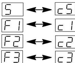
This is how the correcting factor **c** (RTA system) is entered into the circulator. It remains stored in the circulator and is automatically assigned to the corresponding temperature set point.
