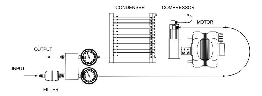
**NOTE:** A filter must always be used. Failure to use a filter will invalidate your warranty.
