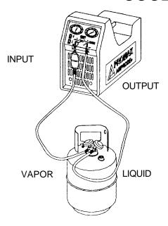
To start you must have a minimum of 2,5 kg of liquid refrigerant in the tank.
