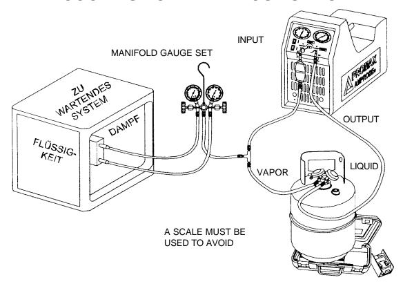
NORMAL RECOVERY: Tank Vapor valve is closed.
